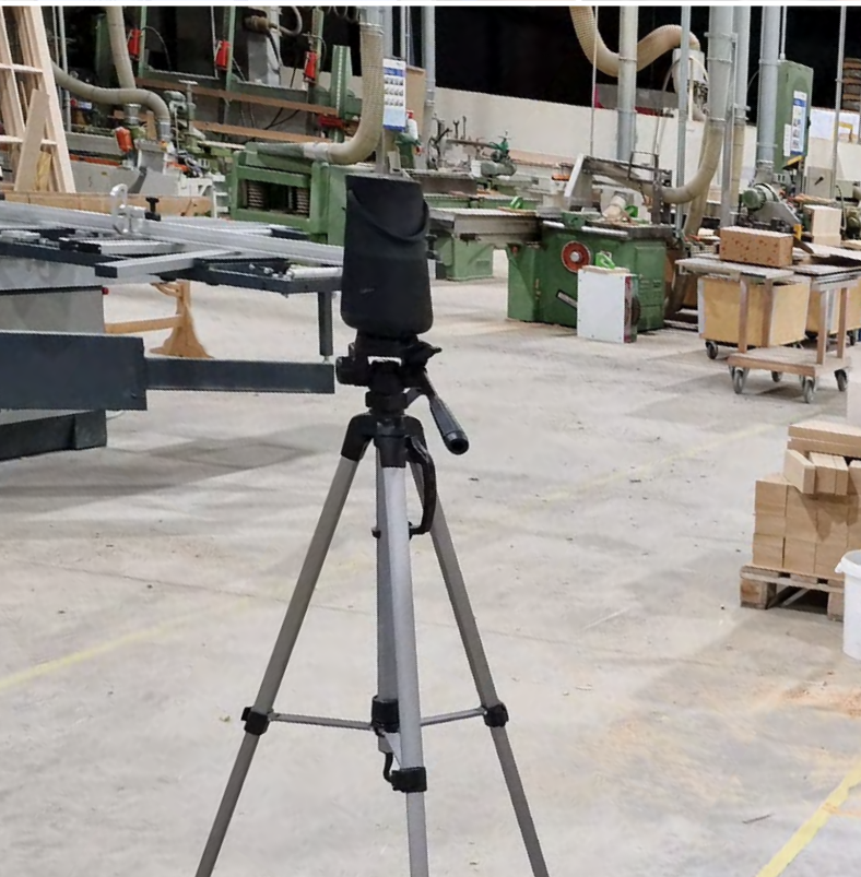
Schallpegeldifferenzmessung Sound measurement
